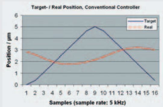
Triangular scanning signal at 312 Hz. There is a significant difference (2.6 μm max.) between target and real position with the conventional PID motion controller.
