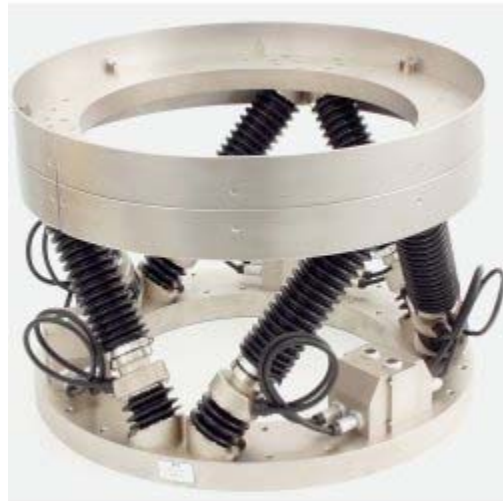
Fig. 15: The waterproof custom-made hexapod for the ALMA telescope.
