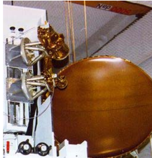
Fig. 13: Two hexapods in a satellite dish reflector and a feed alignment application.
