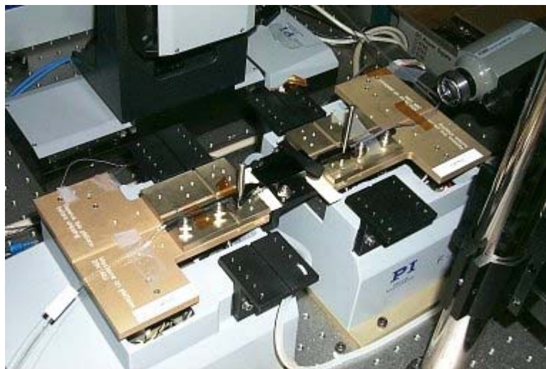
Fig. 18: Two F-206 photonics hexapods in a 12-DOF AWG alignment application. Optical repeatability was found to be better than 0.1 dB.
