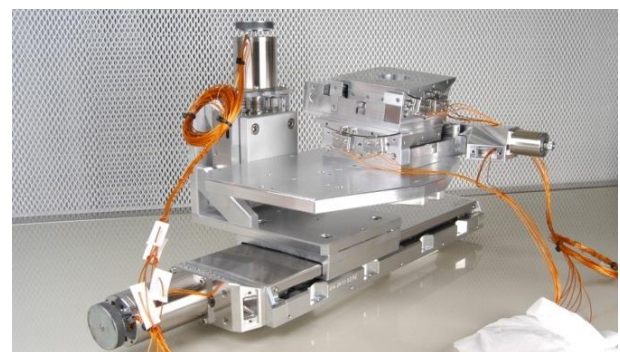
Fig. 2 Four axis system for ultrahigh vacuum application
