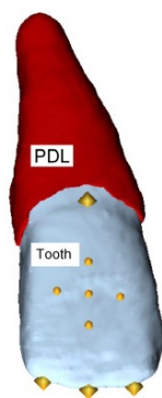
Fig. 4 The tooth reconstructed from radiological data is embedded in the red-colored periodontal ligament (shown without the bone). The loads act on the points shown in the middle portion of the tooth crown as yellow spheres (image: University of Ulm)
