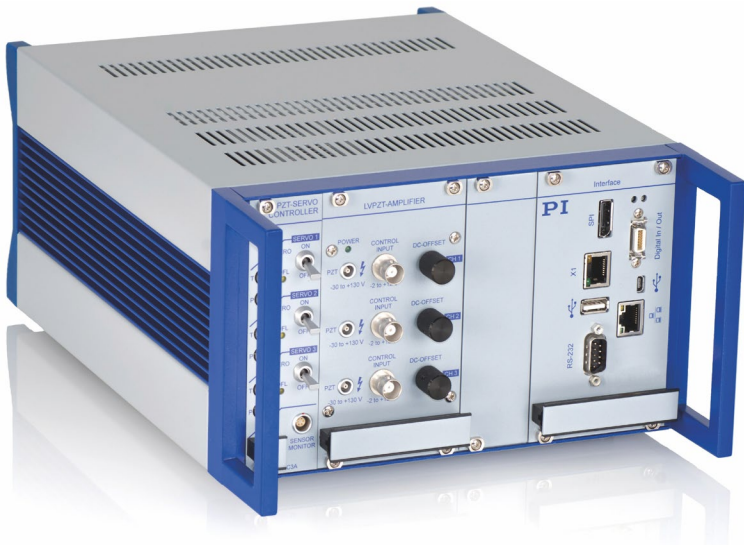
Figure 1: Example of a three-channel system: E-501 housing with E-509 sensor / servo controller module, E-503 piezo amplifier module and E-518 interface module
