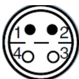
Figure 13: Sensor connection: LEMO connector FFA.0S.304.CLAC32Y, contact side
