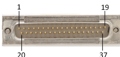
Figure 14: Voltage and sensor connection, sub-D 37 (m)
